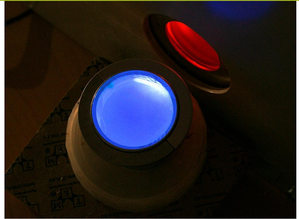
NaI (Tl) scintillator in x-ray beam
