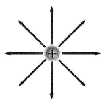
The lines flow out from the positive charge
