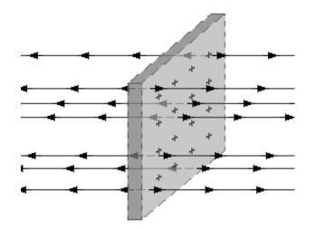
The field lines flow away from the plate on both sides.
