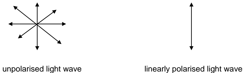
Fig. 4. Spatial system of vectors of electric field intensity for both unpolarised and linearly polarised light observed along the propagation direction of light wave.
