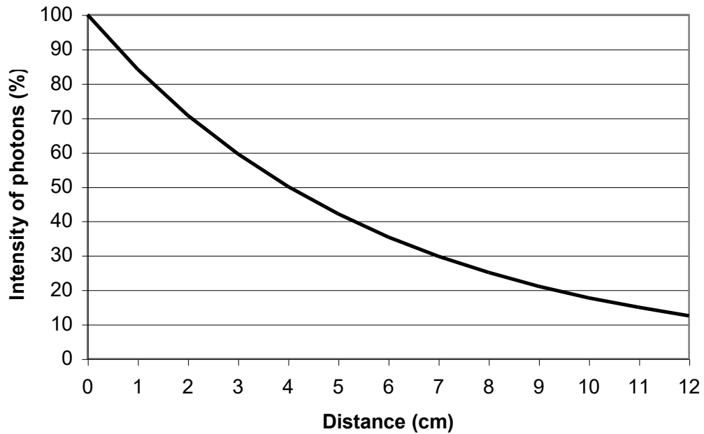
Fig. 6. Percentage changes of intensity of photons \gamma in function of travelled distance in matter
