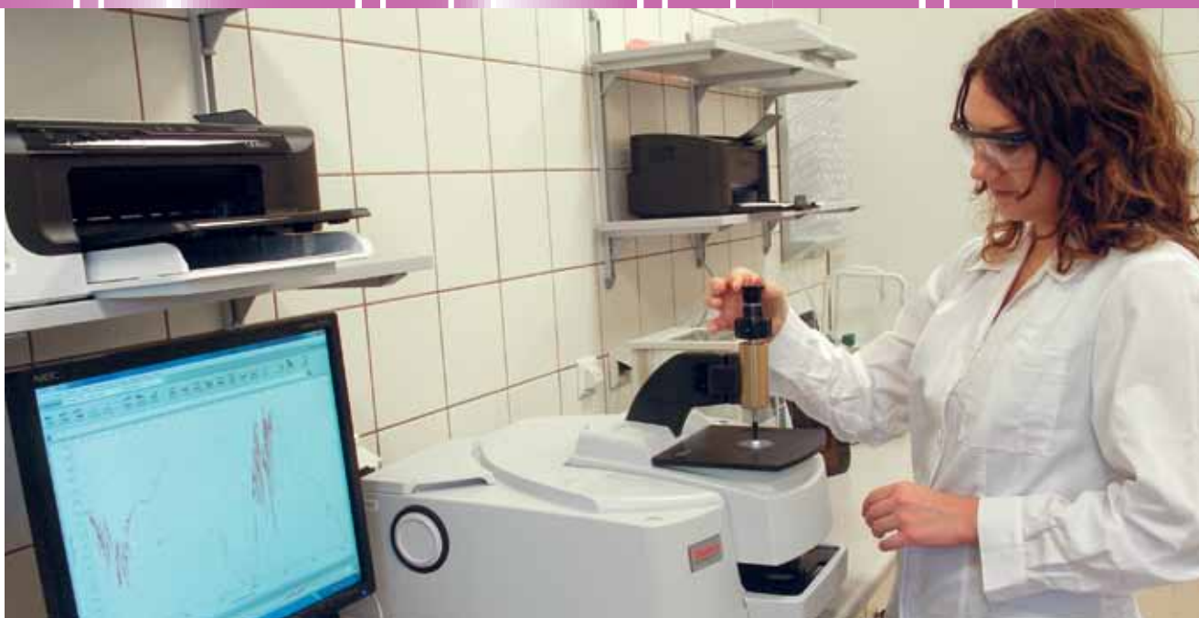
Drug composition analysis by IR spectroscopy
