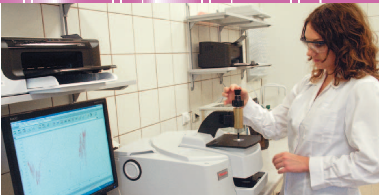
Drug composition analysis by IR spectroscopy
