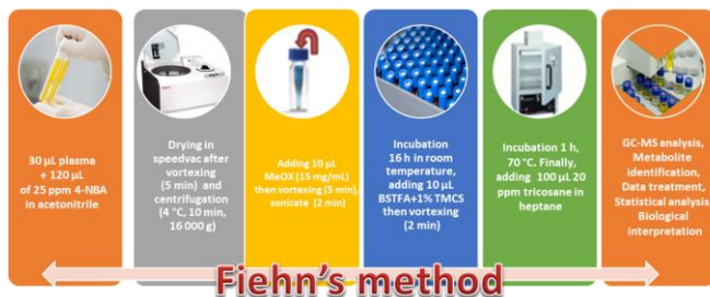
Figure 1. Workflow of plasma sample preparation.
